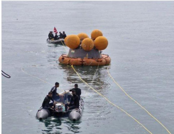
The ISRO carrying out the Well Deck trials of the Gaganyaan missions's crew module in 2024. FILE PHOTO
