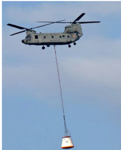
Flight check: The ISRO conducts the first Integrated Air Drop Test for an end-to-end demonstration of the parachute-based deceleration system for the Gaganyaan mission in Bengaluru on Sunday. ANI
