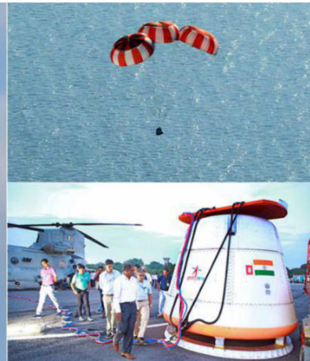
Flight check: The ISRO conducts the first Integrated Air Drop Test for an end-to-end demonstration of the parachute-based deceleration system for the Gaganyaan mission in Bengaluru on Sunday. ANI
