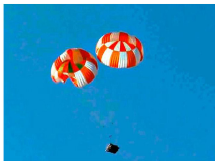
For the Gaganyaan Crew Module, the parachute system comprises a total of 10 parachutes of four types. Photo: X/@isro
