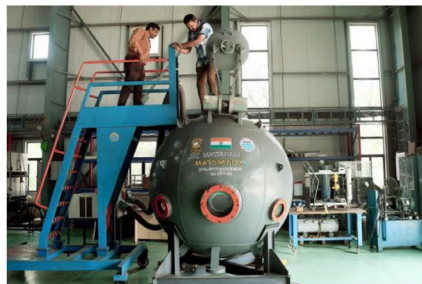
A prototype of the MATSYA 6000, a submersible made by the National Institute of Ocean Technology in Chennai. The final version is expected to undertake a journey to a depth of 6,000 metres. R. RAJENDRAN
